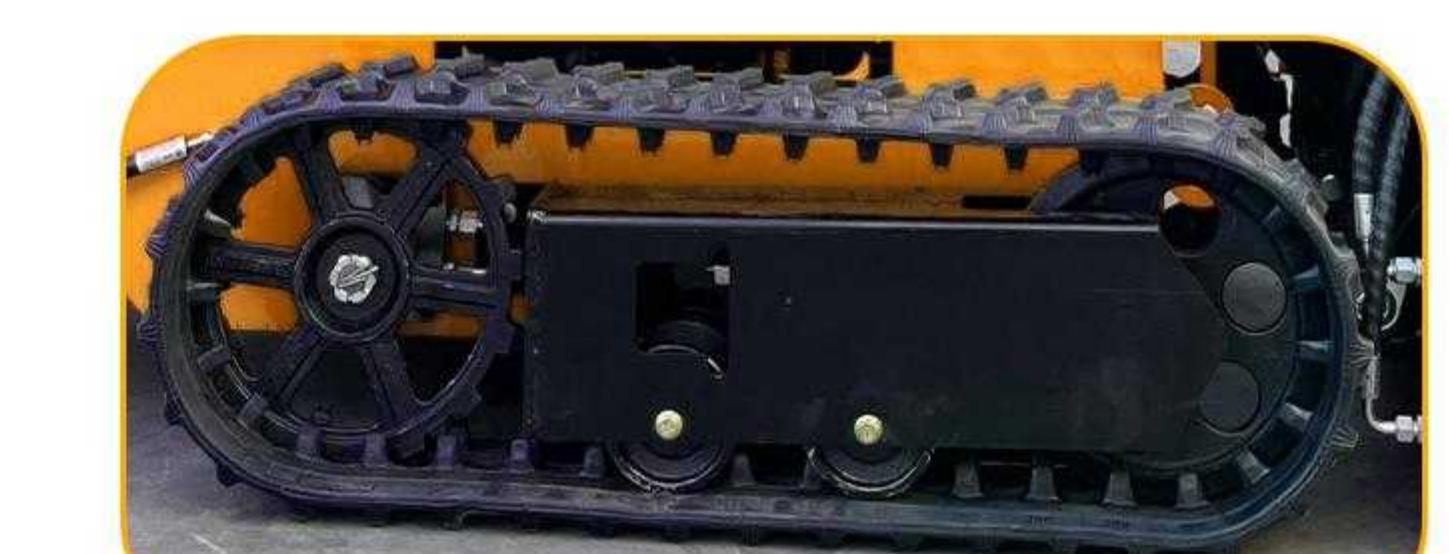
Both wheeled and crawler types use chain drive (four driving force), so the transmission efficiency is higher, and they can work normally in harsh environments. The left and right walking is an independent hydraulics system, and the power is more
