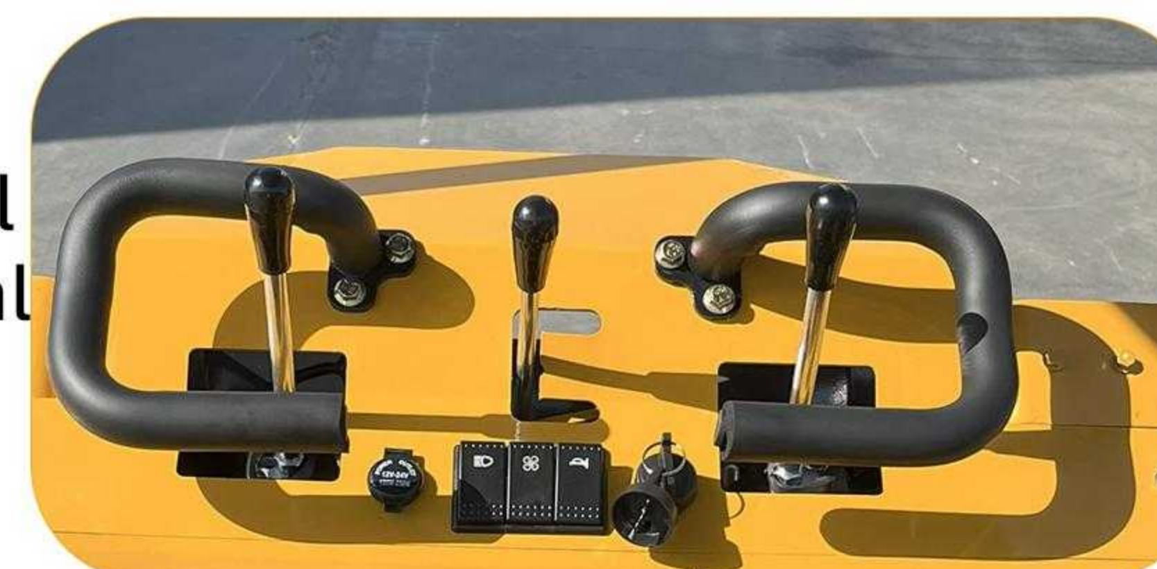
Standard equipped with a double-layer ground control device, featuring an optional joystick, simultaneously operating the drive system and boom, enhancing maneuverability.
